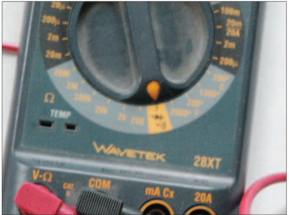
Corrosion can exist where it is not visible – inside the wire casing. Learning how to operate a volt/ohm meter can help you detect this type of wire corrosion easily.
