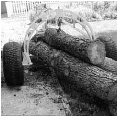
Future Forestry Products has a line of six arches of varying sizes. The arch is wheeled over the log, its cable is slipped under the log, then “chokes” it and picks the log up with a winch “We redesigned it to be effective in carrying all wood, instead of dragging it along,” says Mark Havel.
