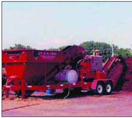
S&S Tree and Horticultural Specialist in South St Paul, Minn., uses a Rotochopper tub grinder to make and color mulch.
