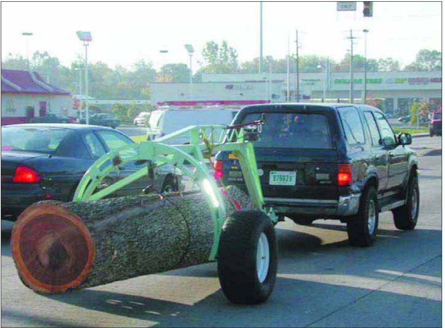
A Future Forestry Products Arch is one way to get a log from a backyard to the sawmill.
