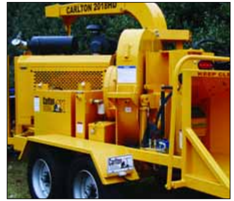
J.P. Carlton makes five chipper models, all disk, mostly using Deutz, Kubota, Caterpillar or John Deere diesel engines.
