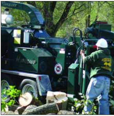
A Morbark Hurricane 18 with CAT 213 hp power unit. Morbark uses mainly diesel in its six models of 8- to 18-inch chippers.
