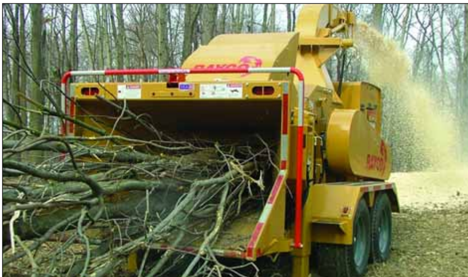
Rayco's RC 20xp 20-inch capacity whole tree drum chipper has a 225 hp turbo-charged John Deere diesel engine that attaches to a maintenance free hydraulic self-adjusting clutch. Automatic feed control protects the engine from overloading and enhances machine performance. Rayco's fuel saver technology throttles the engine down to an idle if the feed wheel control bar is left in neutral for more than 60 seconds, minimizing fuel consumption.
