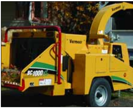
Vermeer's high/low, two-position throttle has a rocker switch the operator can hit to easily adjust engine speed. Introduced in part to lower noise, the switch has evolved into a bit of a fuel miser; making it easy for the operator means they tend to lower throttle more often.
