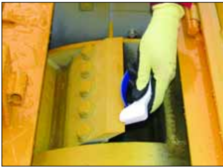
Bandit's design allows users to touch up the chipper knives. "The biggest thing to rob horsepower and drive up fuel consumption in a chipper is dull knives," says Bandit's Jerry Morey.
