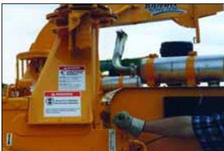
Steps to increase fuel efficiency at Bandit include creating discharge systems, such as this swivel discharge option, that use the natural energy of the chip coming off the knife to assist in the discharge, a design that allows anvils to drop into their proper settings automatically.
